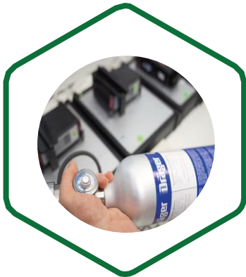
Gas Detector Maintenance and Calibration
